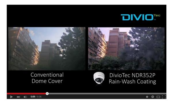
By employing new hydrophobic technology, DivioTec's rain-wash coating is capable of preventing water from attaching to the surface of cameras specially designed for outdoor environments such as parks, parking lots, harbors, etc. In addition, any dirt or dust attached to the cover would be washed away during rainfall or other exposure to water without leaving any water stains or droplets on the cover surfaces.
